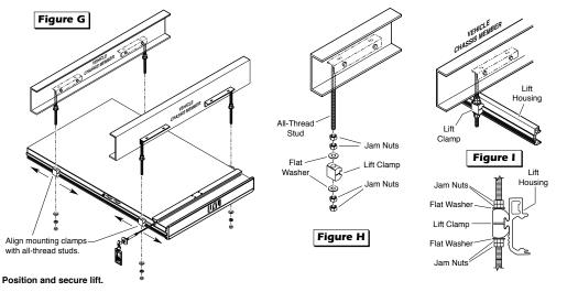
Thread two 3/4" hex jam nuts fully onto each mounting bracket all-thread stud. Place one large diameter flat washer onto each all-thread stud (use tape to hold in place). See Figures G and H
